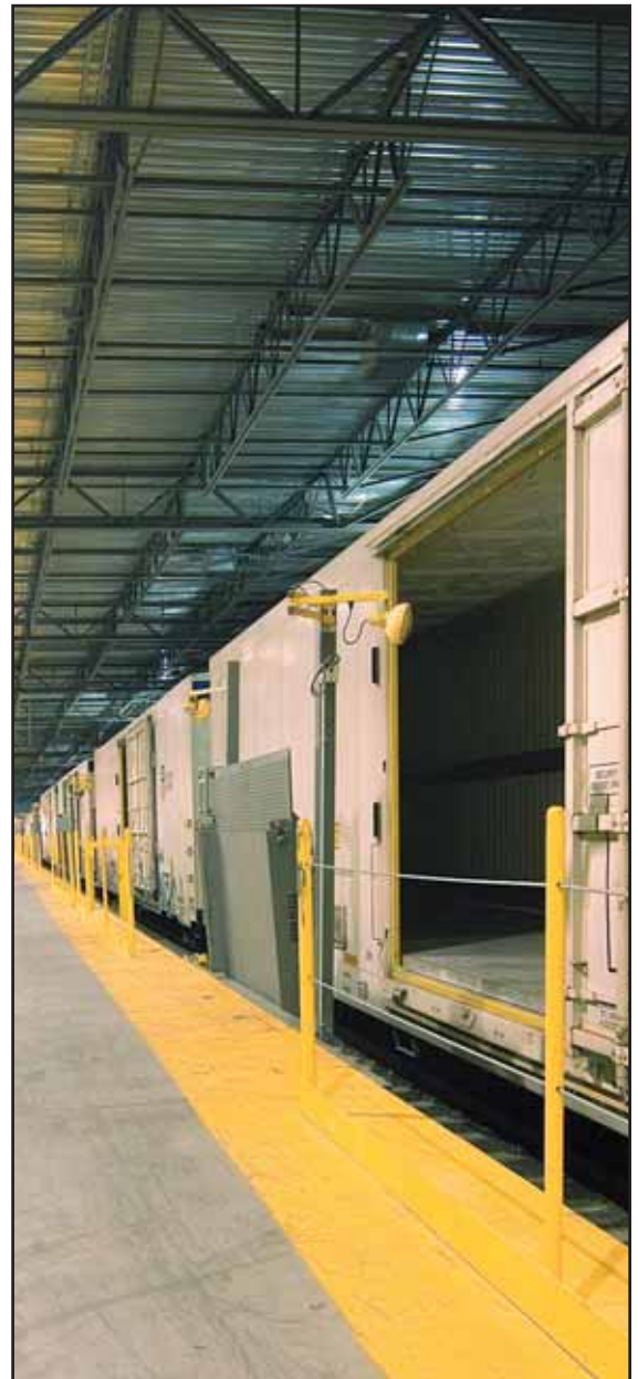
Ready and waiting...part of the 55-car train stands on the mark for loads of Northwest produce inside Railex's Wallula terminal. Each 64-foot long car is temperature and humidity controlled, with GPS equipment so its status can be checked at any time.
